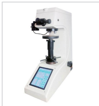
HV-5,10,30,50 (A)T 触摸屏 (自动转塔) 维氏硬度计 (砝码加荷) Touch-Screen (Auto Turret) Vickers Hardness Tester (Weights)
