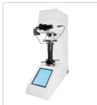
HVS-5,10,30,50 (A) ET 触摸屏数显 (自动转塔) 维氏硬度计 (电加荷) Touch-Screen Digital (Auto Turret) Vickers Hardness Tester (Sensor)
